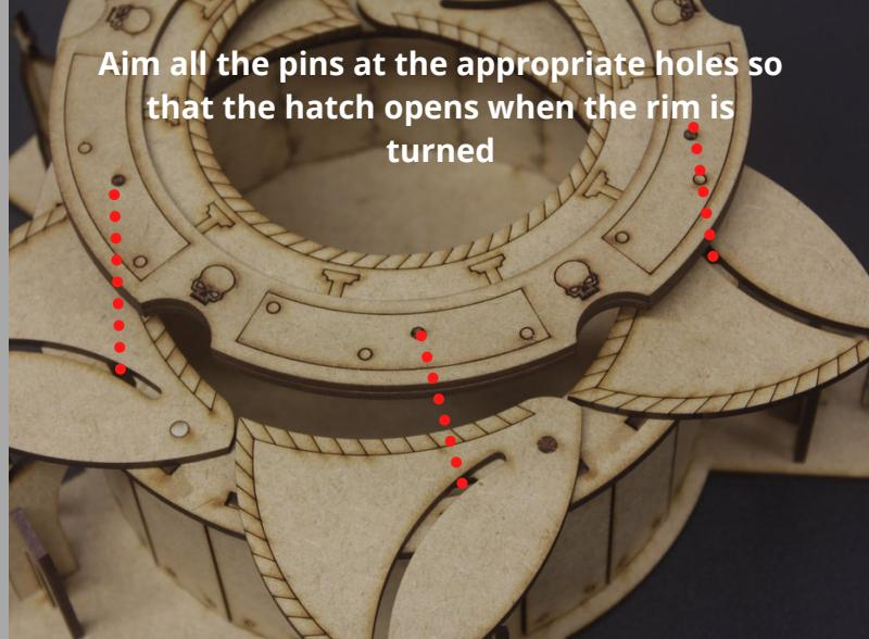
Aim all the pins at the appropriate holes so that the hatch opens when the rim is turned
